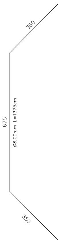
Ⓝ ARMADURA INTERNA PELE BLOCO
